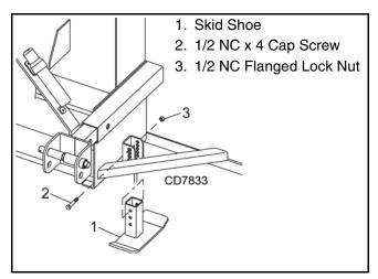
Figure 14. Skid Shoe Adjustment
